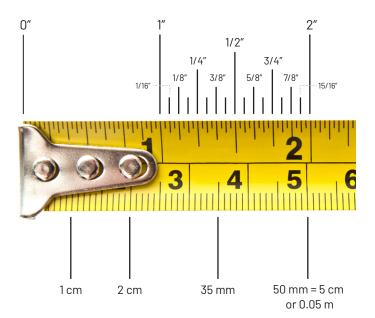
Between each inch marker, there are 15 lines that vary in size depending on what fraction of an inch is the right measurement. The largest marks on the tape are the inch markers, and the number to the left is the inch measurement. The lines decrease in length as the measurement gets smaller, with the smallest line indicating a measurement down to 1/16-inch.
